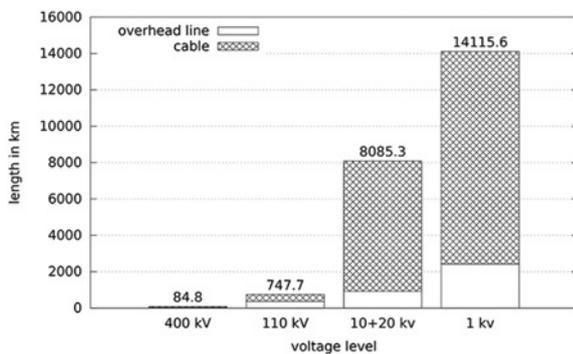
**Fig. 2** Overview line/cable length of Wiener Netze GmbH (as of 2014, [5])
