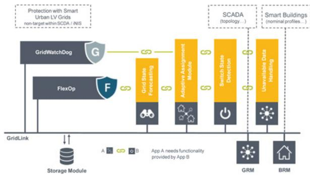
**Fig. 1** Set of applications supporting a P&A approach within an intelligent secondary substation
