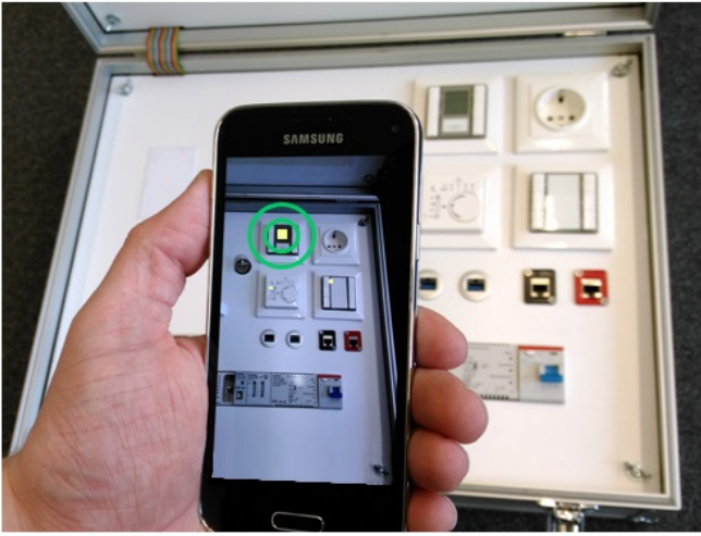
Fig. 2. Smartphone app, that has just identified a component by detecting its light signal emission
